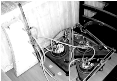
Fig.3 Measurement of heated air with Pitot tube
