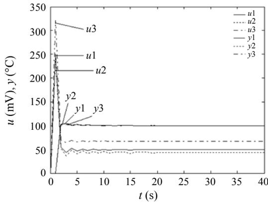
Fig.1 Temperature response curves for three water pipes of a heater
