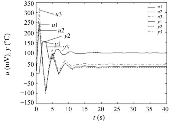
Fig.2 Temperature response curves for three water pipes of a heater with disturbance
