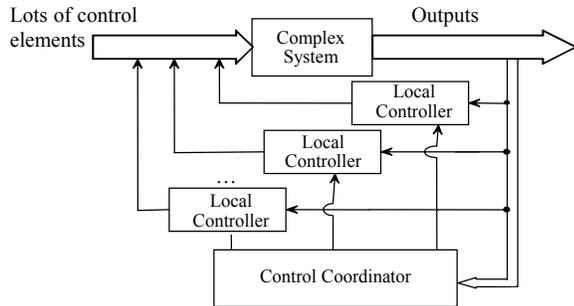
**Fig.1** The diagram of the optimal coordinated voltage control
