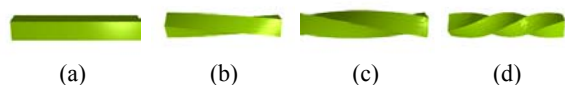
Fig.2 The twist deformation editing of Cube model. (a) The initial model; (b)~(d) The result of twisting 45°, 90° and 110° respectively
