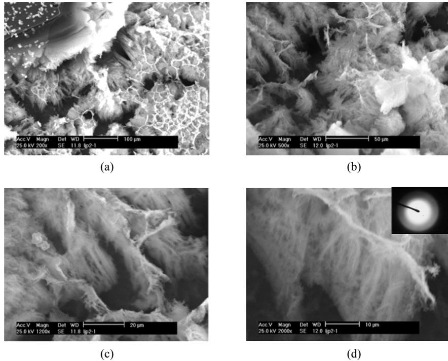
**Fig.1 (a) SEM micrograph of CdS dendrites grown on silicon substrates; (b) Porous structure formed under the compact CdS dendrites; (c) Low magnified SEM images of the oriented CdS/SiO<sub>2</sub> nanowire arrays; (d) High magnified SEM images of the oriented CdS/SiO<sub>2</sub> nanowire arrays, the inset is the selected-area electron diffraction pattern**
