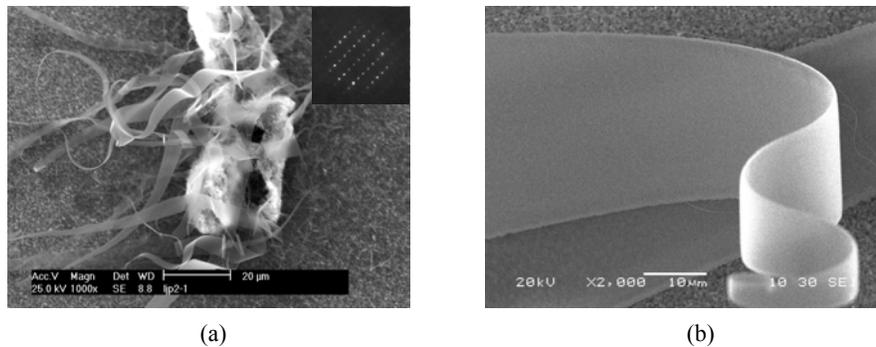
**Fig.2 (a) SEM image of CdS nanobelts, the inset is the selected-area electron diffraction pattern; (b) SEM image of a single CdS nanobelt**
