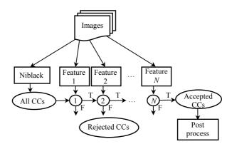
Fig.2 The text detection algorithm
