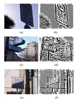
Fig.3 NLNiblack results: black 1, white -1. (a) (c) (e) are original pictures and (b) (d) (f) are the corresponding NLNiblack results
