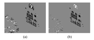
Fig.6 Effect of shape regularity classifiers. (a) Input: edge contrast result; (b) After shape regularity classifiers
