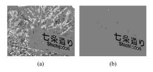
Fig.8 Effect of spatial coherence classifiers. (a) Input: stroke result; (b) After spatial coherence classifiers
