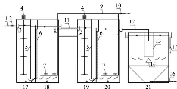
**Fig.1 Schematic diagram of the pilot-scale experimental setup**
