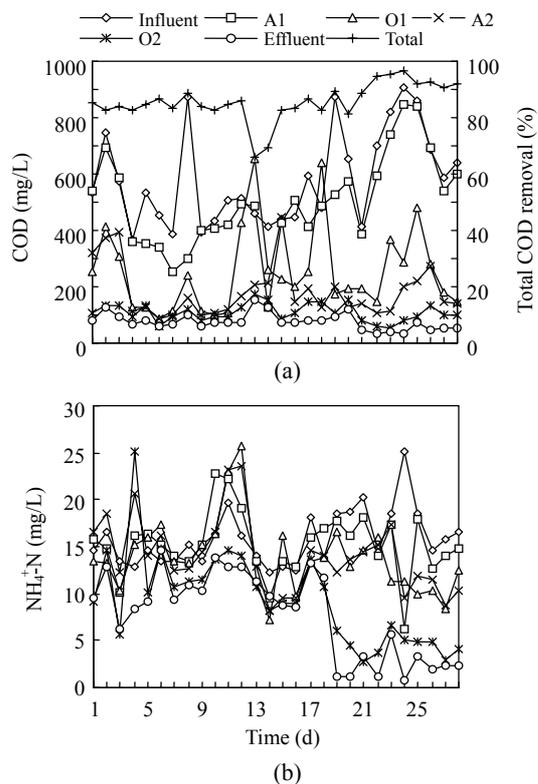
**Fig.5** The daily concentration changes of COD (a) and  $\text{NH}_4^+\text{-N}$  (b) in regular production phase
