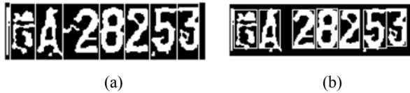
Fig.7 Character segmentation results. (a) The rough split character; (b) Denoised segmentation
