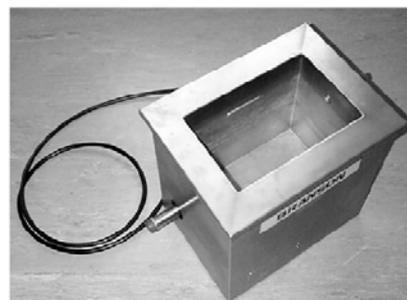
Fig.2 Laboratory ultrasound reactor for reduction of fungi
