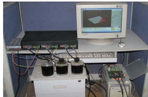
Fig.3 CNC experimental system based on step motor
