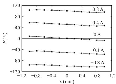
Fig.2 Static force-versus-displacement characteristics
