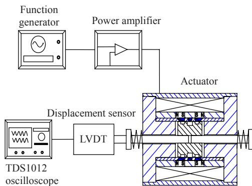
**Fig.4 Schematic of the experimental system**
