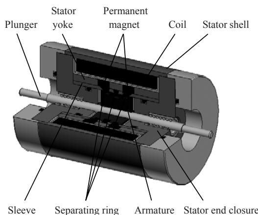
**Fig.1 Structure of the actuator**
