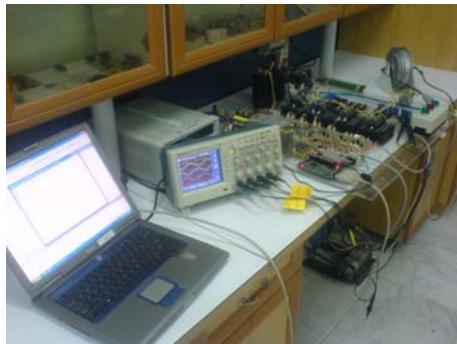
**Fig.4** Experimental setup of the sensorless brushless DC motor drive system
