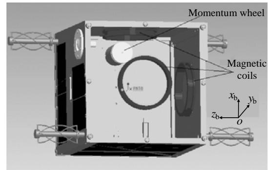
Fig.1 The prototype of the pico-satellite
