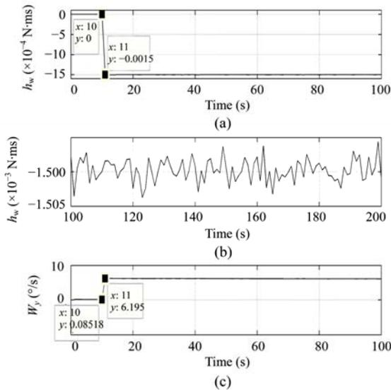
**Fig.3 The momentum wheel start-up process.** (a) Angular momentum of the wheel; (b) Angular momentum instability of the wheel; (c) Pitch angular velocity change during the start-up period
