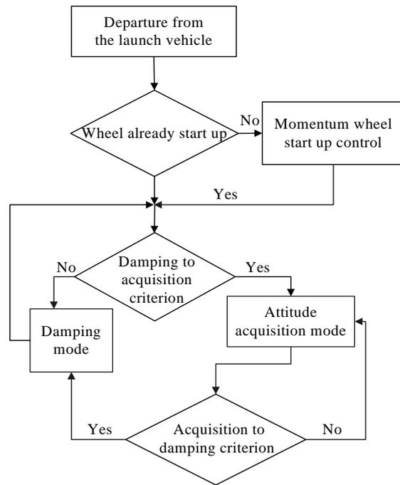
Fig.2 Control flow of the pico-satellite
