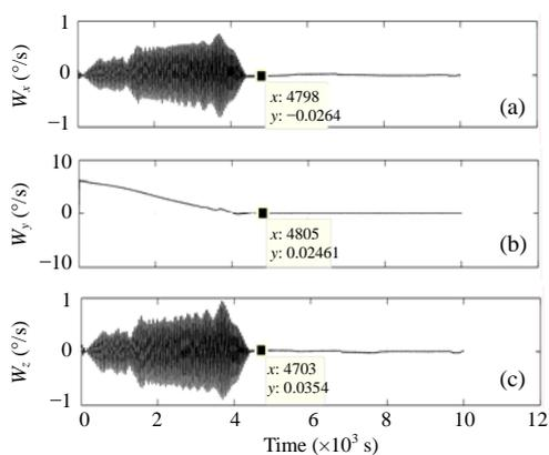
**Fig.7** The variation of attitude angular velocities using combined start-up control. (a) Roll angular velocity; (b) Pitch angular velocity; (c) Yaw angular velocity
