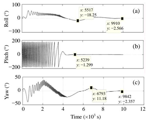
**Fig.6 The variation of attitude angle using combined start-up control. (a) Roll; (b) Pitch; (c) Yaw**
