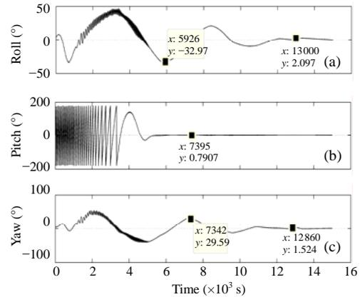
**Fig.4 The variation of attitude angle without wheel start-up control. (a) Roll; (b) Pitch; (c) Yaw**
