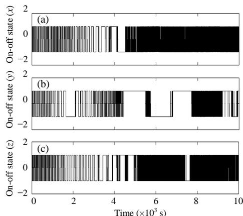
**Fig.8** The operation states of magnetic coils using combined start-up control. (a) Operation state of magnetic coil in  $x_b$ -axis; (b) Operation state of magnetic coil in  $y_b$ -axis; (c) Operation state of magnetic coil in  $z_b$ -axis
