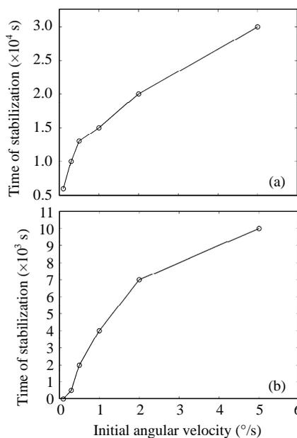
**Fig.9** Time of stabilizing under different initial angular velocity. Wheel starts up (a) after and (b) before separation
