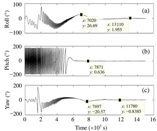
**Fig.5 The variation of attitude angle using wheel start-up control. (a) Roll; (b) Pitch; (c) Yaw**
