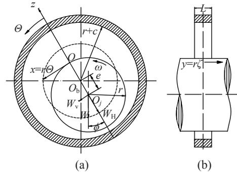
Fig.2 Schematic diagram of self-acting gas-lubricated journal bearings. (a) Cross section; (b) Axial section
