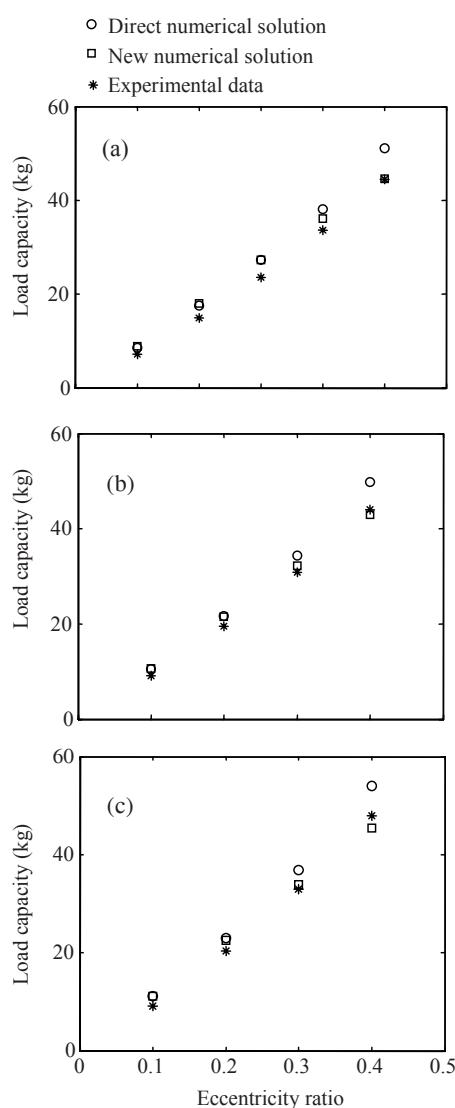
**Fig.4 Comparison of load capacity when the bearing number  $A$  is (a) 1.63; (b) 3.26; (c) 4.89**
