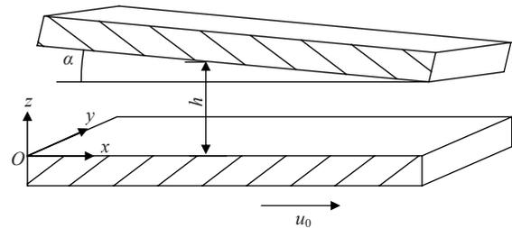
Fig.1 Sketch of gas-lubricated journal bearings' model
