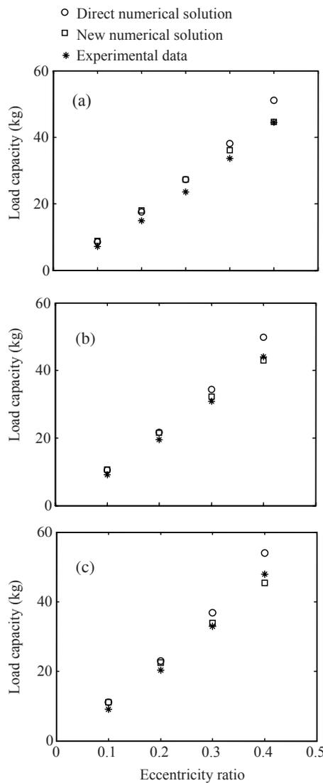
**Fig.4 Comparison of load capacity when the bearing number  $\lambda$  is (a) 1.63; (b) 3.26; (c) 4.89**
