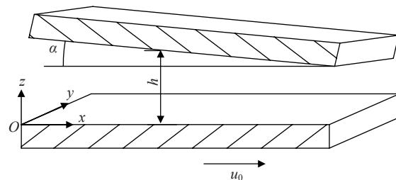
Fig.1 Sketch of gas-lubricated journal bearings' model
