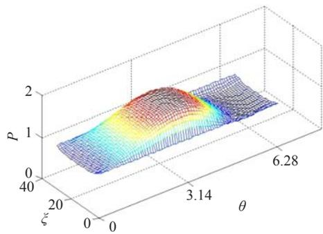
**Fig.3 Non-dimensional pressure distribution of self-acting gas-lubricated journal bearings**
