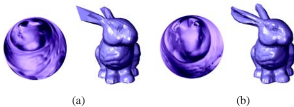
Fig.9 Parameterization and remeshing comparison for the Bimba model. (a) The method of Zayer et al. (2006). In the remeshing result, the two ears have been under-sampled; (b) Our method
