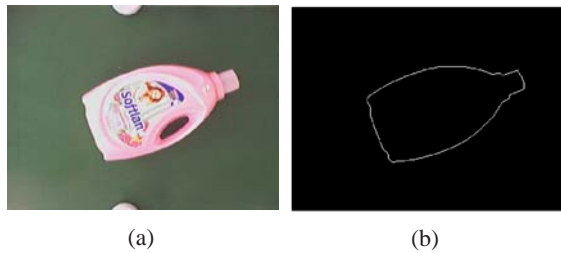
Fig.2 (a) An example of a digitized image as it is taken by the Webcam; (b) The binarized edge of the object after pre-processing
