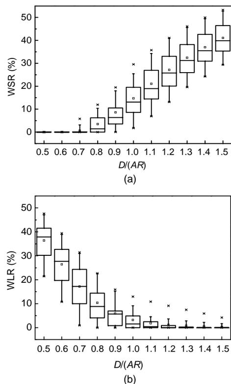
Fig. 6 Distributions of WSR (a) and WLR (b) under various conditions of ratios of  $D/(AR)$  when  $S/(AR)=0.8$
