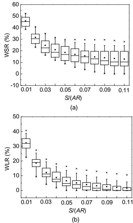
Fig. 5 Distributions of (a) WSR and (b) WLR under various conditions of storage capacity when  $D/(AR)=1$ . The boxes extend from the 25th percentile to the 75th percentile, with a line at the median. The whiskers show the 5th and 95th percentiles. Small star represents the highest and the lowest values and the small diamond represents the median value (50th percentile)
