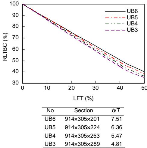
Fig. 9 Behavior of RLTC of a family of long span beams with  $L_E/D=30$
