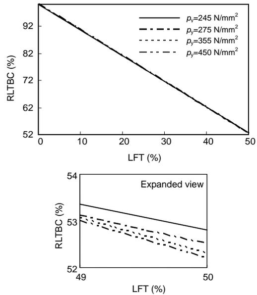
Fig. 6 Effect of design strength on the RLTBC of a corrosion damaged beam (UB60)
