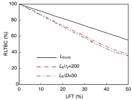
Fig. 11 Minimum curves for estimating the RLTC of corrosion damaged beams
