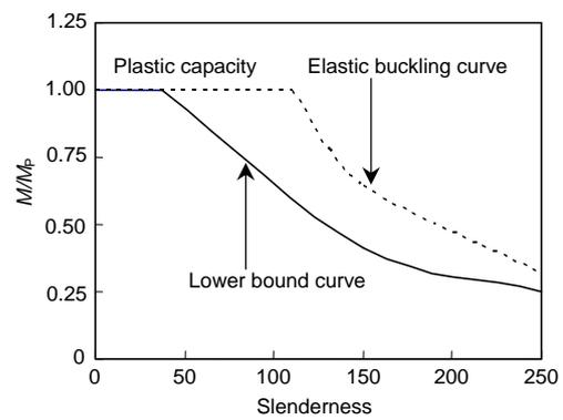
Fig. 4 Lateral torsional buckling behavior of a beam
