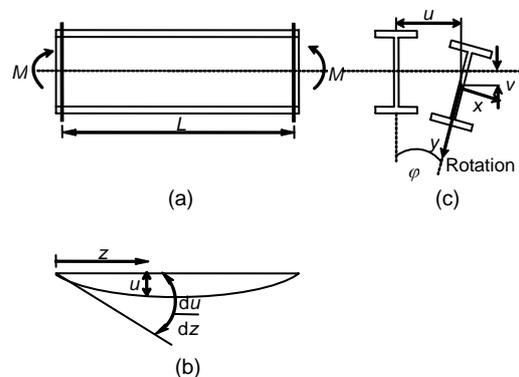
**Fig. 3 Lateral torsional buckling of a simply supported I-beam. (a) Elevation; (b) Plan on the longitudinal axis; (c) Section**
