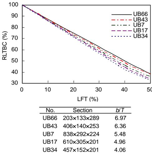
Fig. 10 Behavior of RLTC of long span beams from five families
