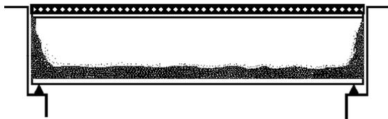
**Fig. 1** Typical locations where corrosion can occur on a steel girder bridge (Kayser and Nowak, 1989)
