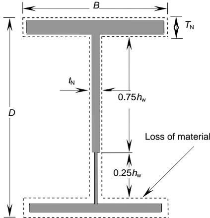
**Fig. 2 Varying thickness loss model**
