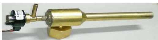
Fig.3 Adjustable ejector with nozzle needle
