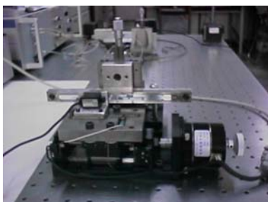
Fig. 9 A photo of the assembled dual positioning stage
