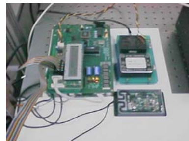
Fig. 6 Optical encoder with the signal processor
