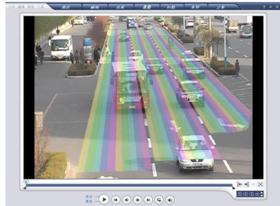
Fig. 1 Video image of lateral separation distance survey in Weixing Road, Changchun City, China
