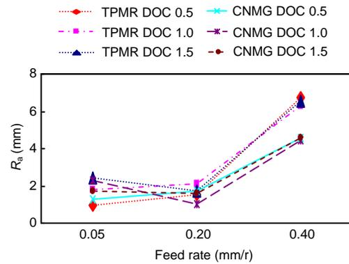
Fig. 3 *R<sub>a</sub>* plot of TPMPR versus CNMG at a cutting speed of 150 m/min (DOC 0.5: depth of cut 0.5 mm)
