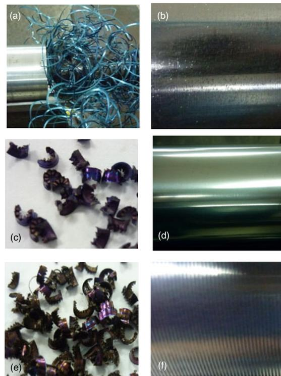
**Fig. 5** Chips formed and surface roughness resulting from each feed rate
