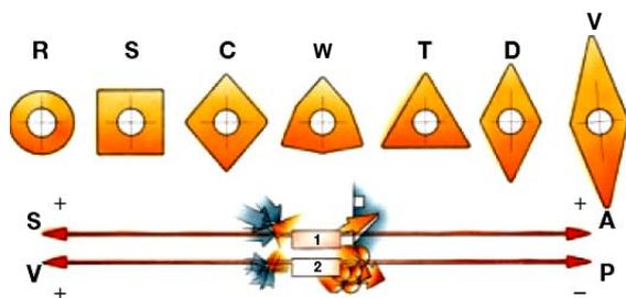
Scale 1 indicates that as regards cutting edge strength (S), the larger the point angle to the left, the higher the strength. While as regards versatility and accessibility (A), the inserts to the right are superior. Scale 2 indicates that the vibration tendency (V) rises to the left while power requirement (P) is lower to the right
