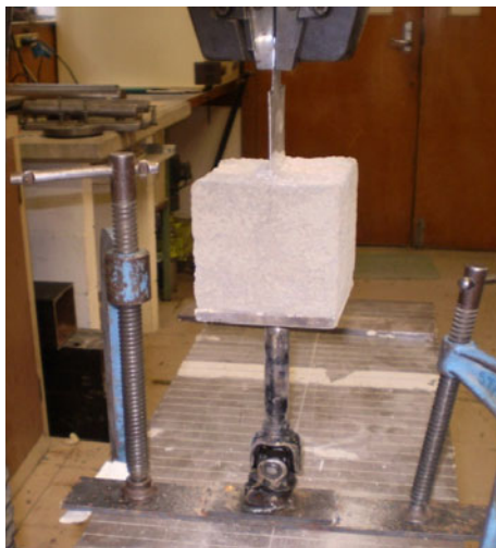
Fig. 2 Testing mechanism with a freely adjustable ball-joint and a plate with embedded-bolts within cement-based material samples
