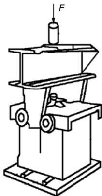
Fig. 3 Test set-up of WS specimen (DL/T 5332-2005, 2006)
