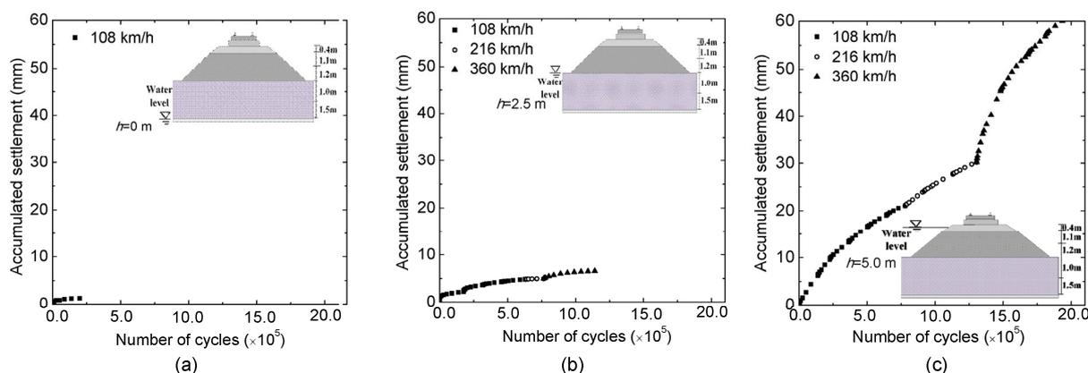
Fig. 3 Accumulative subgrade settlement under different water levels (Chen *et al.*, 2014a): (a) water level is at the bottom of the foundation; (b) water level is at the top of the foundation; (c) water level is at the top of the subgrade
