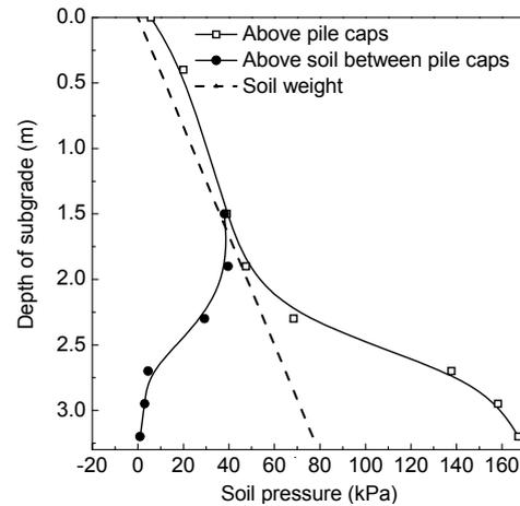
Fig. 1 Static soil pressure in the subgrade (Chen *et al.*, 2014c)
