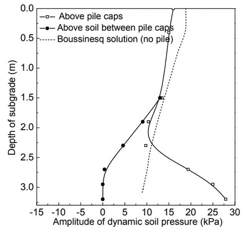
Fig. 2 Dynamic soil pressure in the subgrade (Chen *et al.*, 2014c)
