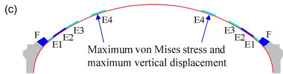
**Fig. 16 Vertical displacement and von Mises stress of the steel liner at the construction stage E4**
