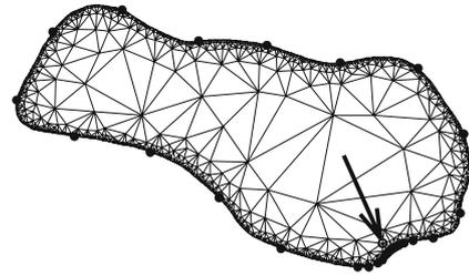
**Fig. 3 Adaptive triangle mesh constructed over the cloned region (from Fig. 1a), and hierarchical boundary sampling result (dots on the boundary) of the inside vertex (pointed out by an arrow). The same strategy from Farbman *et al.* (2009)**
