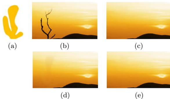
**Fig. 5** Hiding the tree in the scenario of sunset with the patch image. (a) The patch image with pure color; (b) Original (target) image; (c) Poisson cloning; (d) MVC cloning; (e) Harmonic cloning. Note that the results of Poisson cloning and harmonic cloning are nearly the same. The shadow-like pattern in (d) is produced because the MVC membrane in each branch region is affected by values along the boundary of each other, despite there being no straight sight between the two branches
