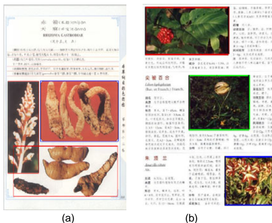
Fig. 4 Image separation results on a page with one (a) and more than one (b) column using the gray histogram projection method
