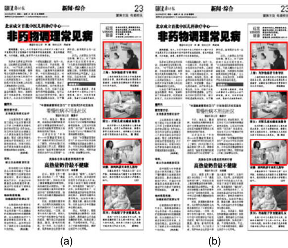
Fig. 5 Image separation performance of the region growth method without (a) and with (b) combining the Ada-Boosting algorithm
