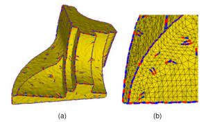
Fig. 4 Feature directions of detected feature vertices. In (a) each initial feature vertex is shown in color. Feature direction and its opposite direction are shown in different colors. (b) is the zoom-in view of part of the model
