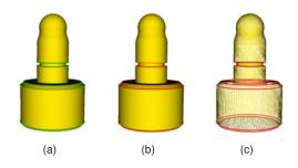
Fig. 7 Detected feature vertices (a) and feature lines (b and c) of a machanical bin
