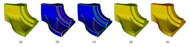
Fig. 1 Method overview. (a) is the initial feature vertex detection on a noisy Fandisk model. Sharp edge and corner type vertices are shown in different colors. (b) and (c) are the color maps of salient measure before and after weak feature enhancing, respectively. The weak features at the top of the fan are marked by an ellipse. (d) and (e) are the final detected feature vertices and feature lines, respectively
