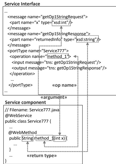
Fig. 5 Matching between the service interface and the service component
